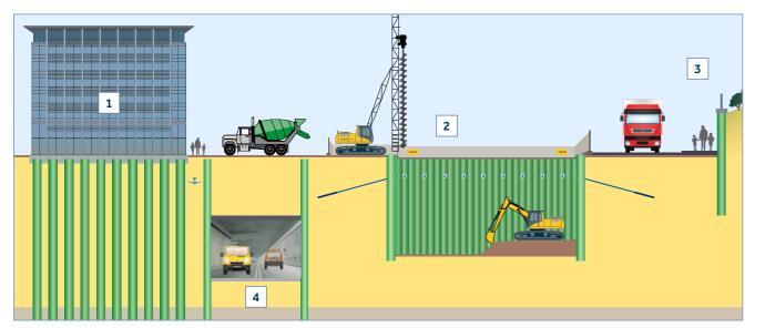
1. Foundations CFA piles are extremely effective at providing structural support for a range of structures such as buildings by transferring loads into the underlying soil.
